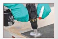
Our range of machines and diamond core-bits offers ideal solutions for drilling, before and after installation, porcelain tiles and slabs (even 3 mm thick), single and double fired, marble, granite, natural stones, etc. ... up to a maximum diameter of 120 mm (4 3/4''), starting from 6 mm (1/4''). From the super-professional drilling machines, ideal for a comfortable and simple drilling up to simpler solutions, but certainly not less effective, such as humid use diamond bits.
